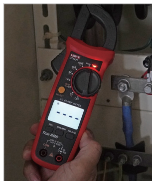
NCV multi-segment display and audio/visual alarm
