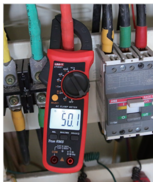
High voltage (600V) frequency measurement
